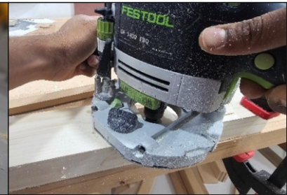
Use a flush trim bit in router machine for smoothing joint
