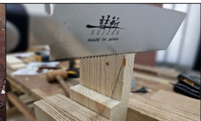
Use rip hand saw for cutting the dovetail joint
