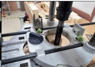
Use 16mm trim bit in router machine grooving the Pillar
