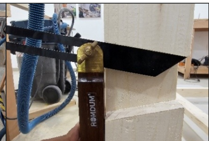
Set the bevel square with Pillar for marking
