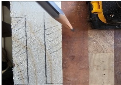
Marking for T-bridle joint in top rail
