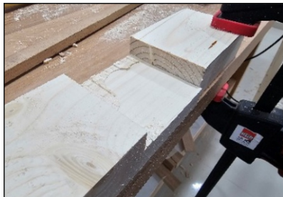
Use f-clamp for chiselling the joint
