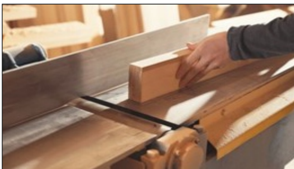
Surface planing at 90-degree angle
