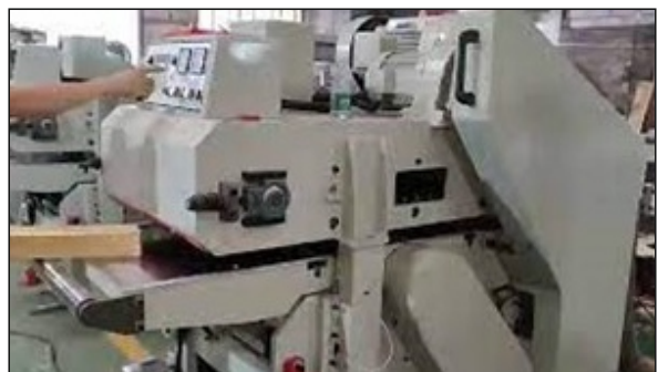
Thickness planing in accurate required size
