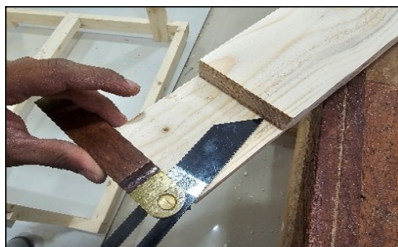
Make on the side bottom rail by using bevel square
